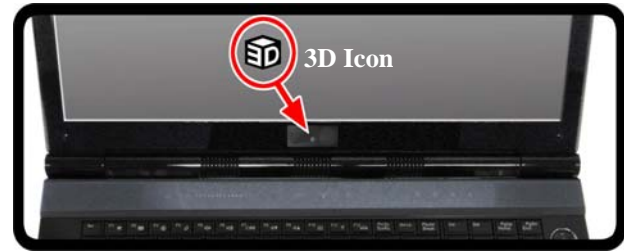
Figure 12 - IR Emitter Location
