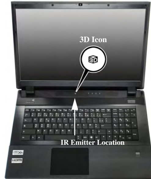
Figure 12 - IR Emitter Location
