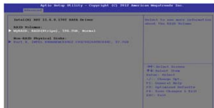
Figure 4 Informations RAID (Advanced > Intel(R) Rapid Storage Technology)
