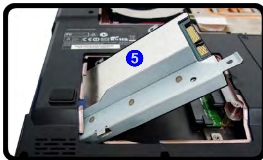
Figure 6 - 9 Secondary HDD Assembly Removal (Model C)
