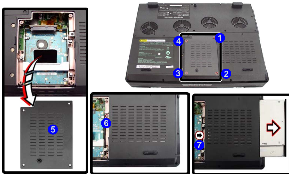
Figure 6 - 13 Removing the CD/ DVD Device(s)
